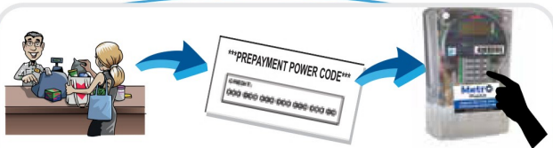
When a power code is purchased, the code is printed on a cash slip or sent by text. This power code is then keyed into the secondary meter and the meter is recharged.
